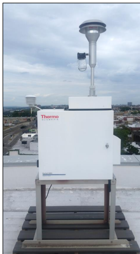
Figure 2-2 Filter-Based PM 2.5 Sampler in Union City
